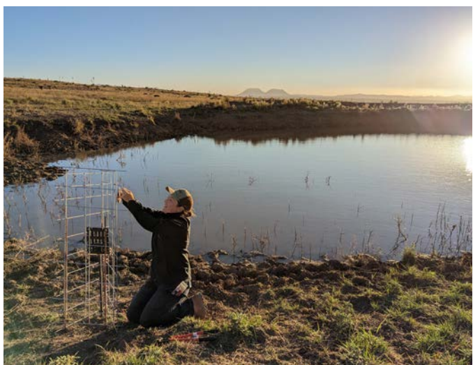
Image 2: Autonomous recording units were mounted next to dirt livestock tanks and protected with cattle panels. (photo credit: Emily Blumentritt/BRI)
