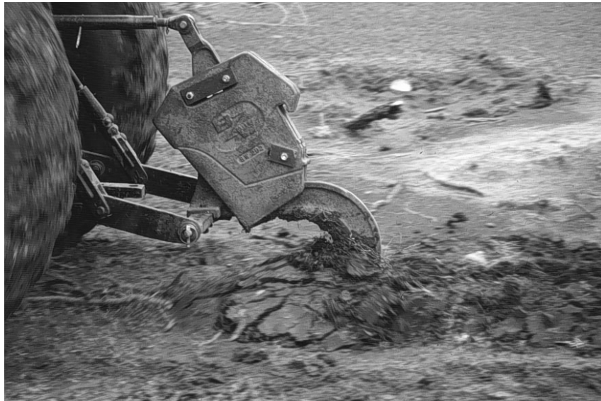
Figure 2. Single-shank ripper used for restoration of a clay loam range site near Carlsbad, Texas in 1995 and 1996.
