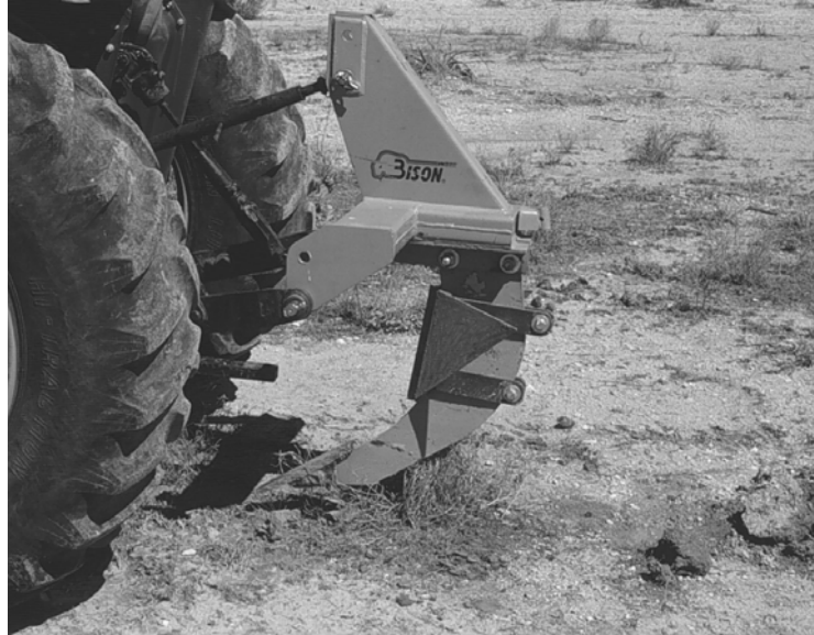
Figure 7. A single-shank ripper (Bison SVH-1, Bison Equipment Co., Waco, TX) with shop-made wings.
